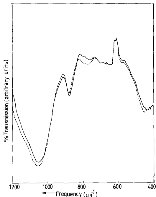
Figure 5 Spectra of a 77 mol% SiO 2 -23 mol% CeO 2 thin film (—) before and (---) after annealing.
